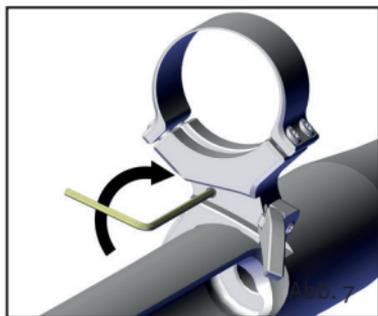
7. Secure the threaded spindle with the grub screw with a hex key wrench 1,5mm.
